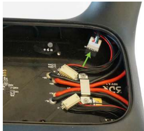
Figure 10.4.3.1: Compass Connector on Mainboard
