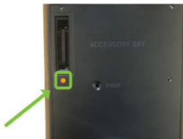
Figure 10.7.2: Strobing Pairing Light
