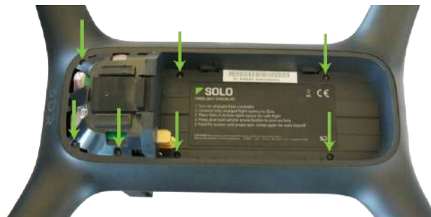
Figure 10.5.2.1: Battery Tray Removal
