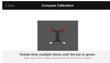
Figure 10.2.1.2: App - Compass Calibration Procedure
