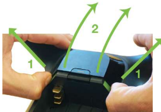
Figure 10.5.1.1: GPS Cover Removal
