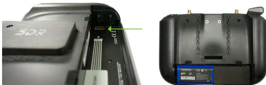
Figure 10.1.1: Controller Battery Installation
