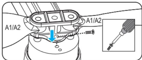
3.1 Unscrew the screw and remove the fan blade.
