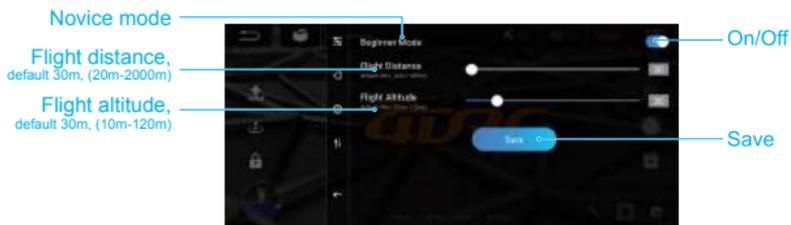
**⚠ Note:** After being proficient in flight operation, it is necessary to close the novice mode and set the flight distance and altitude before the aircraft can fly further!
