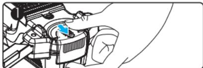
5.1 Buckle the battery lock of the aircraft.
