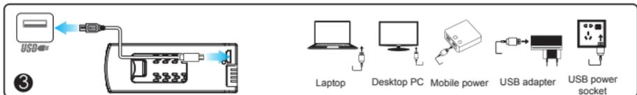
5.3 Charging: Insert the USB port of the USB charging cable into the computer USB port (or use 5V $\Rightarrow$  2A power adapter), and connect the other end of the USB charging cable to the battery socket. When charging, the red indicator on the module battery is on, and when the battery is fully charged, the red indicator light goes out, which means that the charging is complete.
