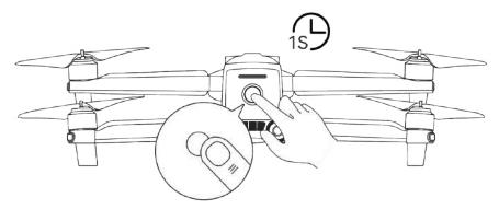
Fig 5-3 Checking Battery Level
