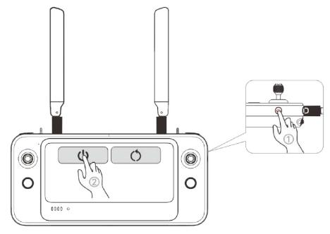
Fig 4-6 Turning the Remote Controller Off
