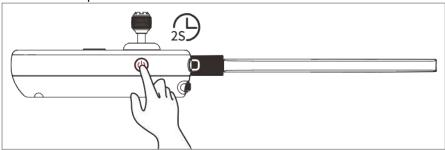
Fig 4-5 Turning the Remote Controller On
