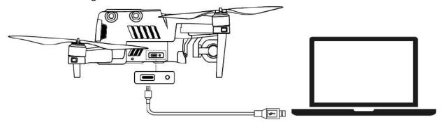
Fig 3-16 Connect the aircraft to PC/MAC
