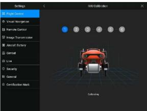
Flip the aircraft 180°, placing it with the belly facing up on a flat surface, until the App prompts you to
