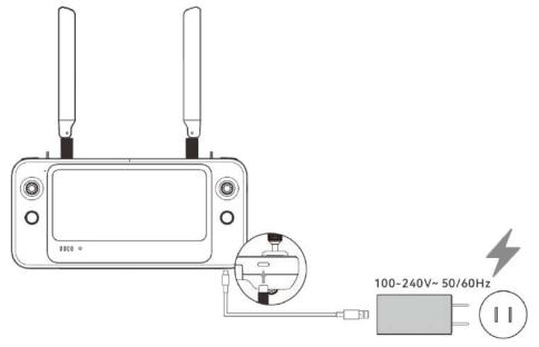
Fig 4-8 Use the RC charger to charge the remote controller
