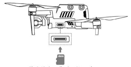
Fig 3-15 install microSD card
