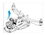
Fig 3-13 Removing the Gimbal
