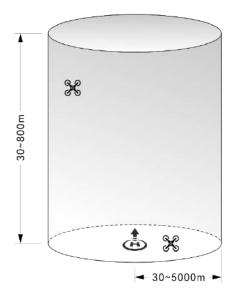
Fig 2-4 Altitude and Distance Limitation Diagram
