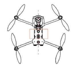
Fig 2-1 Recommended mounted area (bottom view)
