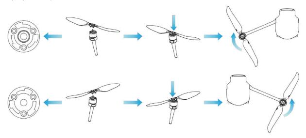
Fig 3-7 Install the Propellers
