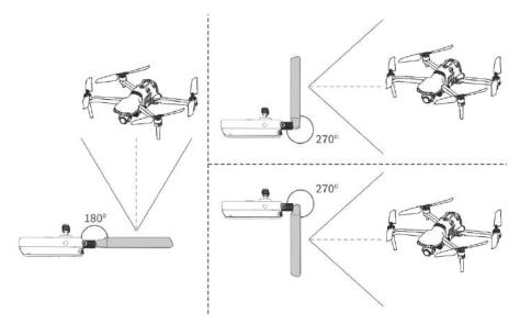
Fig 4-9 Extend the antenna
