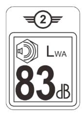
Fig 3-17 A-weighted sound power level of EVO II Pro V3 aircraft
