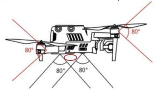
Fig 2-2 Recommended mounted location (not affecting the observation range)
