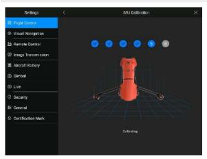
Fold the arms of the aircraft and place it with the nose facing upward on the ground u ntil the App prompts that the calibration is successful. Please be careful to protect the lens on the rear of the aircraft during this process.
