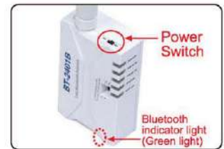
4.1.4 Turn on the power switch (to position ON) of 2.4G Bluetooth Datalink. The green light of bluetooth will flash quickly, waiting for the connection with the phone bluetooth.
