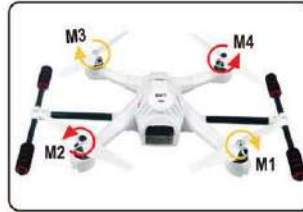
3.3 Propellers assembled (assembled skid landing)
