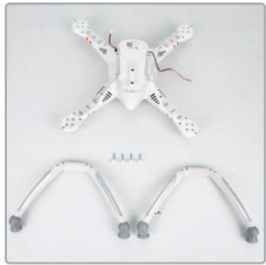
1.1 Prepare quadcopter landing gear and 4 screws.
