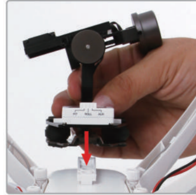
3.2 Slide the gimble onto the mounting track, push on the base until it is all the way back.
