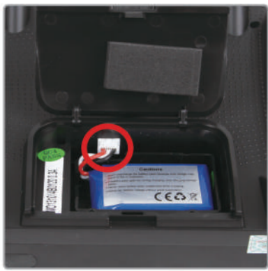
5.1 Connect the battery to the radio. For safety: Make sure the battery is fully charged before you fly!
