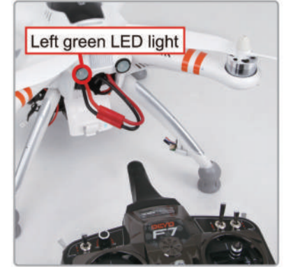
6.6 The left green LED flash quickly till light out which means calibration finished. Please reconnect the aircraft power after calibration.
