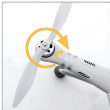
2.2 Match the concave part on the propeller to the concave part on the brushless motor. Match the arrow on the arm to the arrow on the propellers. Double check, this is important.
