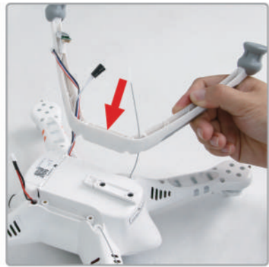
1.2 Install the right skid, carefully pull the cables and the antenna through the holes in the landing gear.
