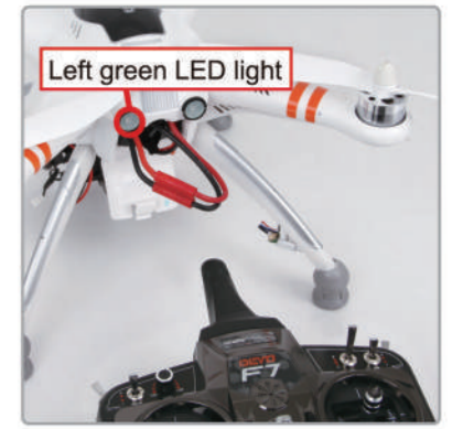
5.4 When the LEFT indicator light stop flashing, the binding is successful.
