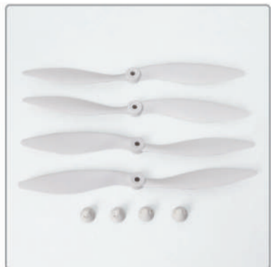
2.1 Prepare 4 propellers and the rounded "nuts", these are called "Spinners".
