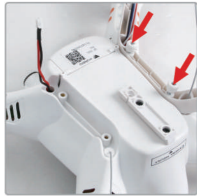
1.3 Secure the landing gear with 2 screws, tighten firmly with your fingers, do not use tools.
