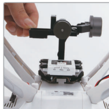
3.3 Done, the gimble is installed.
